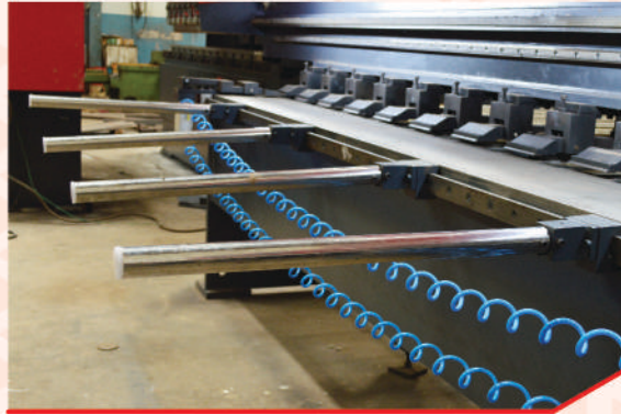
TILTABLE FRONT SUPPORT - 4 NOS.
